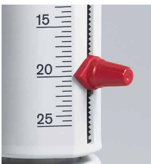
Positive volume setting using interior scalloped track
